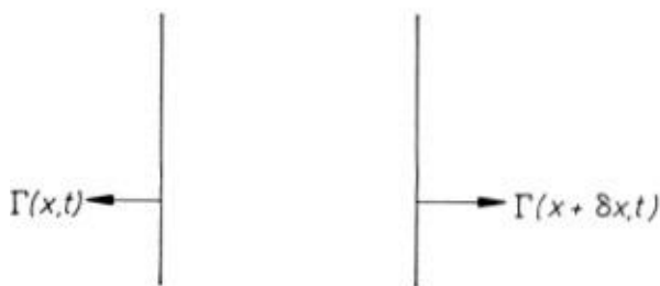
(b) The force per unit area acting on the region is denoted by \Gamma(x, t)
