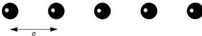
Fig. 2.3 A chain of identical masses M connected by springs: (a) at equilibrium spacings x_n^0 = na ; (b) at displaced positions x_n = na + u_n
