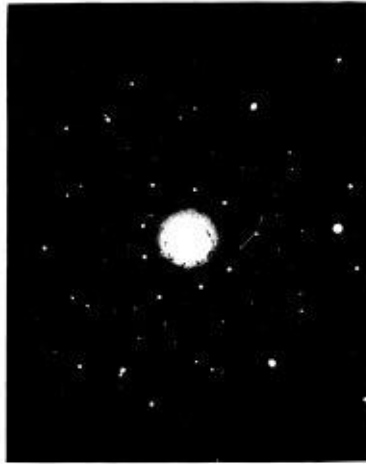
(b) A Laue photograph of Si with a (1 1 1) face normal to the x-rays; note the three-fold symmetry. (Reproduced with permission from Elements of X-ray Crystallography by Leonid V. Azaroff. © 1968 McGraw-Hill Book Company Inc.)
