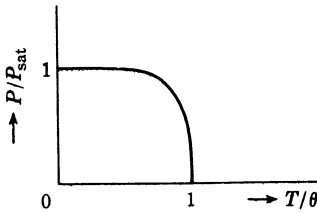
Fig. 8-10. Schematic representation of the spontaneous polarization as function of temperature, as derived from the procedure given in Fig. 8-9.
