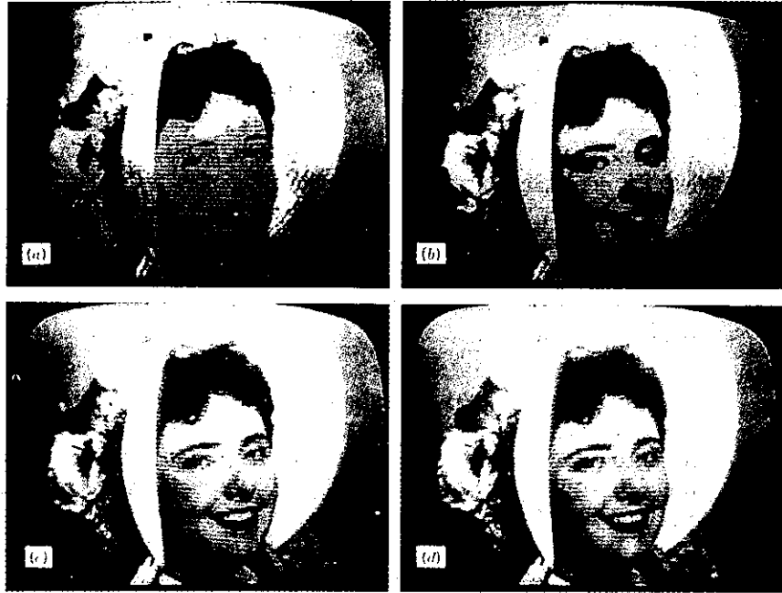
FIGURE 13-9 Television received via PCM. (a) 4 standard levels; (b) 8 standard levels; (c) 16 standard levels; (d) 32 standard levels. (By courtesy of Dr. J. S. Mayo, Bell Telephone Laboratories.)
