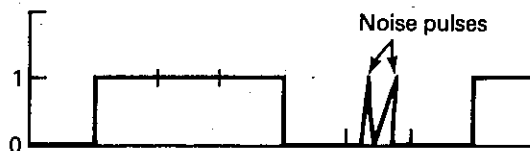
FIGURE 14-17 Data stream with noise pulse.
