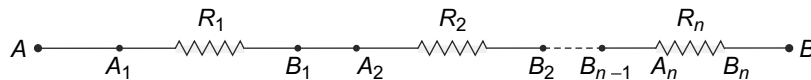
Fig. 5.13 Series combination of n resistances R_1, R_2, \dots, R_n . The ends of the resistances are connected in such a way so as to leave A and B free as the free terminals
