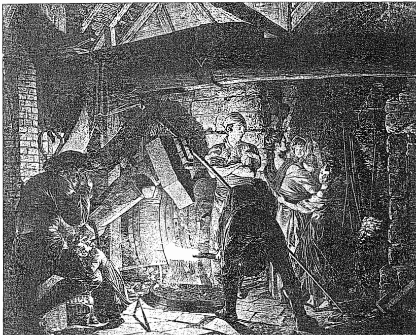
An Iron Forge , by Joseph Wright of Derby, 1772: a family setting. An artist's representation of a 'model' iron-founder with a water-driven tilt-hammer to save effort in the swing of the hammer. Fashion makes its presence felt here too.
