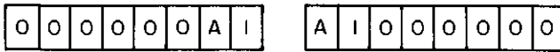
Figure 2.26 Identifier A1 right and left justified and zero filled (6 bits per character)
